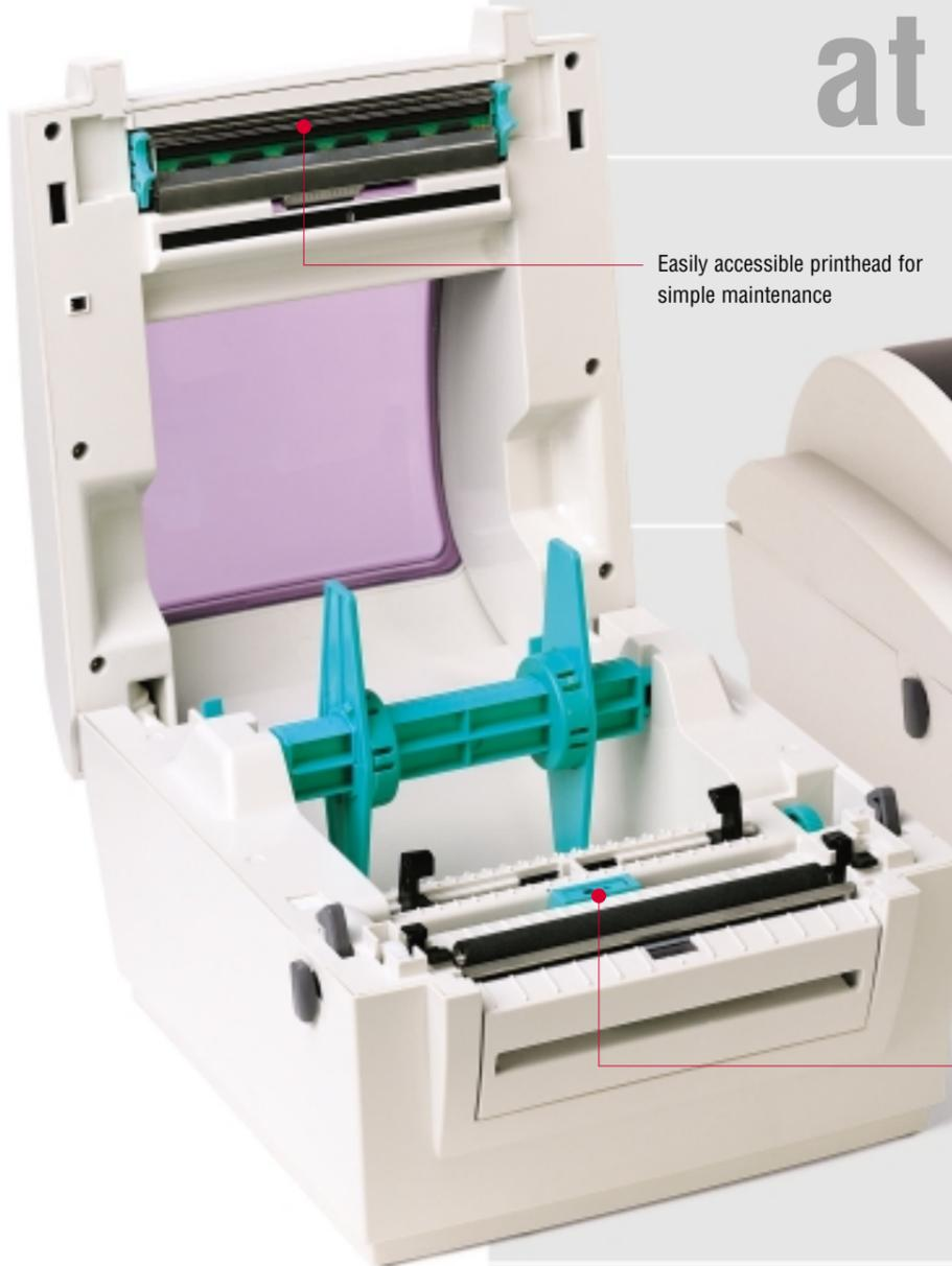
Easily accessible printhead for simple maintenance
