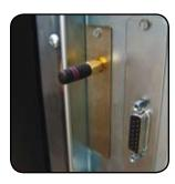
ZebraNet Internal Wireless Plus installed on a Zebra XillIPlus printer
