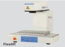
open system with 2 Axis support (Z = 180mm, X = 240mm), comfort operation panel, Laser class 4.
