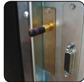
ZebraNet Internal Wireless Plus installed on a Zebra *Xi*IIIPlus printer
