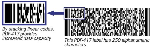
By stacking linear codes, PDF-417 provides increased data capacity.
