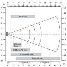
\* The reading distances given are typical reading distances measured in an office environment (200 lux) with extended reading range activated where applicable.
