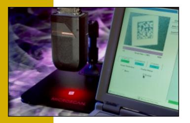
**IP65 Enclosure Rating:** Quadrus' internal circuitry and components are protected against harsh industrial environments by a die-cast aluminum housing which is sealed to IP65 standards (industrial rating for dust and moisture protection).
