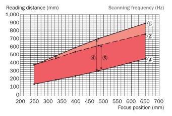
① = Max. reading dist. (aperture angle 25°); ② = Max. reading dist. (aperture angle 50°); ③ = Min. reading dist.; ④ = DOF  $\alpha$  = 0°; ⑤ = DOF  $\alpha$  = 45°
