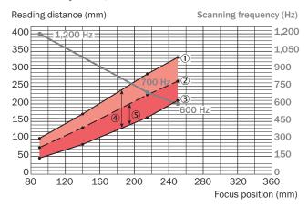
① = Max. reading dist. (aperture angle 25°); ② = Max. reading dist. (aperture angle 50°); ③ = Min. reading dist.; ④ = DOF  $\alpha$  = 25°; ⑤ = DOF  $\alpha$  = 50°
