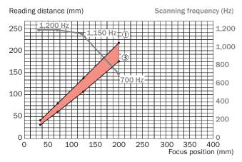
1 = Max. reading dist. (aperture angle 25 °); 3 = Min. reading dist.
