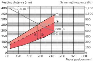
① = Max. reading dist. (aperture angle 25°); ② = Max. reading dist. (aperture angle 50°); ③ = Min. reading dist.; ④ = DOF  $\alpha$  = 25°; ⑤ = DOF  $\alpha$  = 50°
