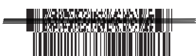
Aim the single scan line at the center of the 2D portion
