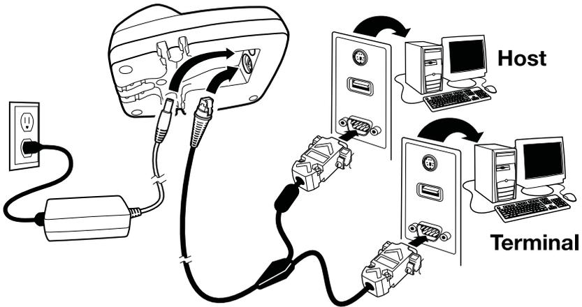
4. Plug the serial connector into the serial port on your computer. Tighten the two screws to secure the connector to the port.
