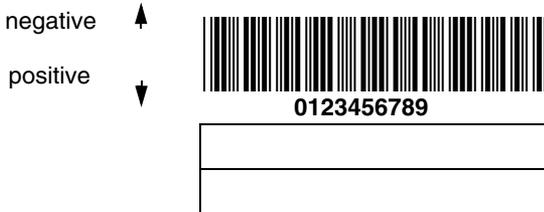
An important aspect of intelligent signature capture is that all dimensions used in the application are measured as multiples of the minimum element size of the barcode. Using this method, intelligent signature capture always outputs the correct image size and resolution, no matter the distance at which the image scanner is held from the barcode, assuming that the entire signature capture area is within the image scanner's field of view.
