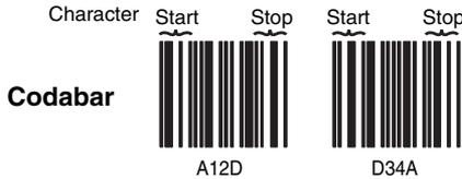
Select Require to prevent the image scanner from decoding a single “D” Codabar symbol without its companion. This selection has no effect on Codabar symbols without Stop/Start D characters.
