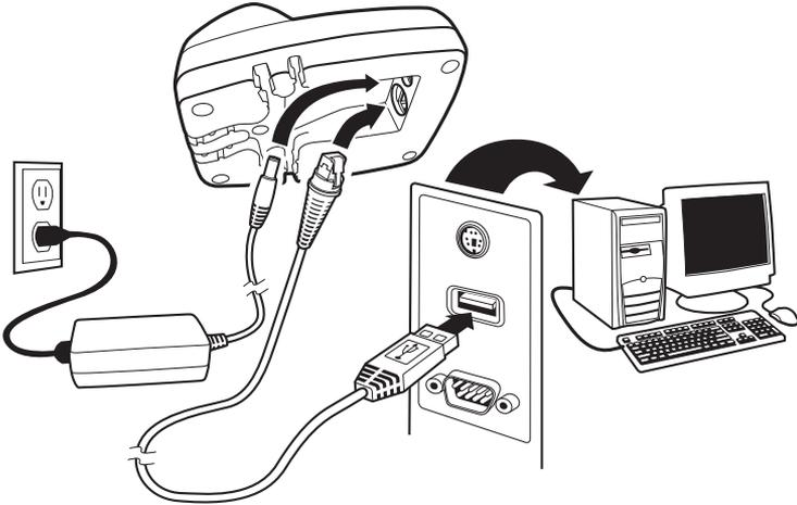
2. Program the base for the USB interface by scanning the appropriate programming barcode See [page 2-5](#).
