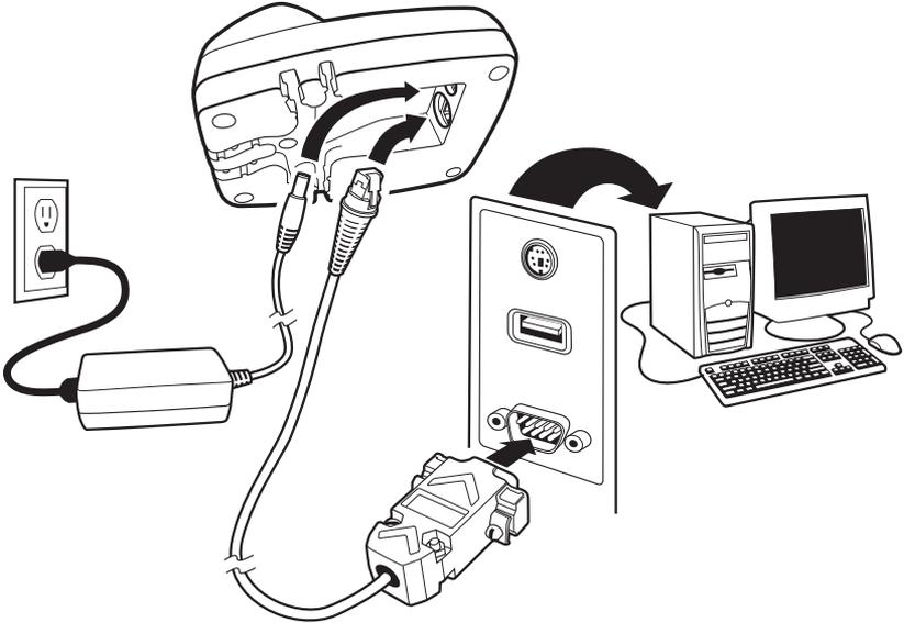
3. Plug the serial connector into the serial port on your computer. Tighten the two screws to secure the connector to the port.
