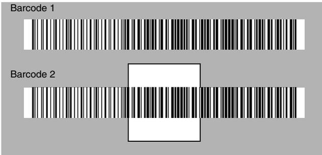
The default centering window is a 128x96 pixel area in the center of the image scanner's field of view. The following diagram illustrates the default top, bottom, left, and right pixel positions, measured from the top and the left side of the image scanner's field of view, which is 640 by 480 pixels.
