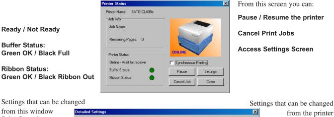
from this window Print Speed Label Size Print Starting Point Correction Print Darkness Darkness Level Zero Slash Paper Specification Proportional Pitch Offset (Mode) Other Size Buzzer
