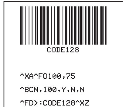
Fig. B: Subset B - With Start Character
